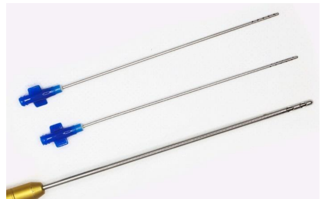
Figure 1: The three cannulas we used for this study. From the top to the bottom: cannula 2 mm, 15 side port holes, 1 mm diameter; cannula 2 mm, 15 side port holes, 0.8 mm diameter; cannula 3 mm 2 side port holes, every hole width 2.5 mm height 5mm (liposuction cannula).
